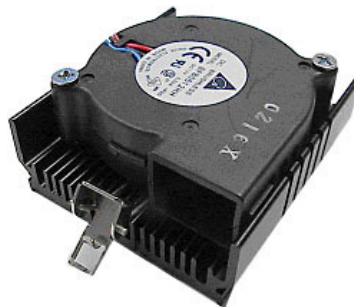
Active Cooler For Intel Pentium® III Socket 370 FCPGA and FCPGA2 (up to 1.4 GHz)
